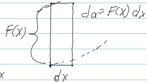
$$3) \quad \bar{x} = \frac{\int x F(x) dx}{\int F(x) dx} = \frac{\int_0^2 x[-x^2 + 2x] dx}{\int_0^2 (-x^2 + 2x) dx}$$
