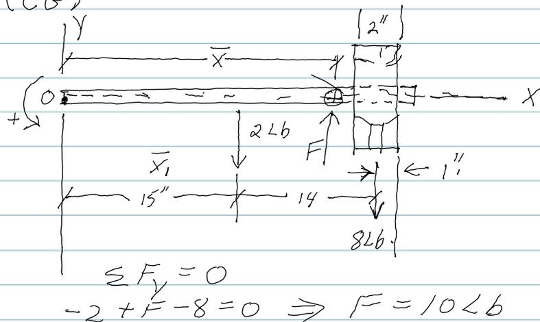
$$\bar{x} = \frac{F_1 \bar{x}_1 + F_2 \bar{x}_2}{F_1 + F_2} = \frac{\sum_{n=1}^i F_i \bar{x}_i}{\sum_{n=1}^i F_i}$$
